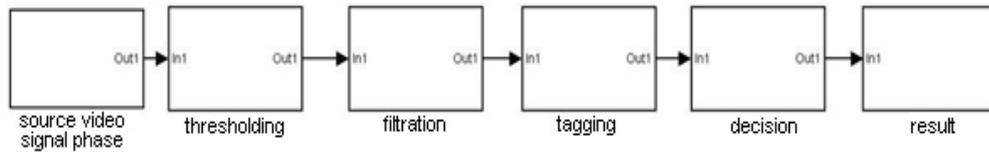
Figure 5-Block Diagram of Interferogram Video Signal Analysis Program
